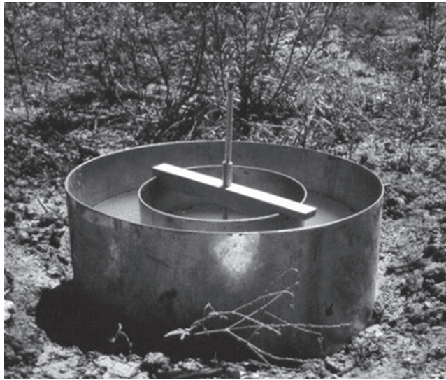
Fig. 5.3 Double-ring infiltrometer. (Reproduced with permission of Eijkelkamp Agrisearch Equipment BV, Giesbeek, The Netherlands.)
