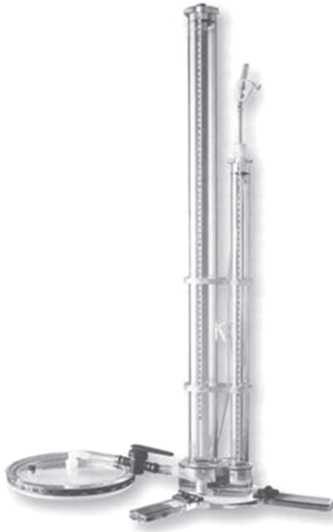
Fig. 5.8 A tension infiltrometer. Reproduced with permission of Soil Measurement Systems.
