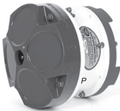
Fig. 7.14 An acoustic Doppler current profiler (ADCP) showing the transducers. (Reproduced with permission of Teledyne RD Instruments.)
