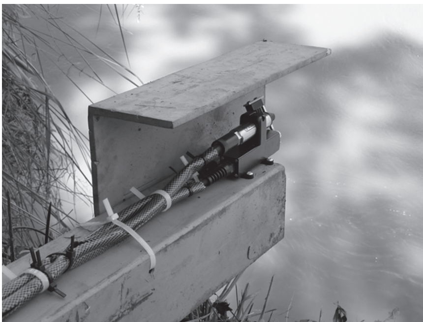
Fig. 8.5 An OBS-3+ turbidity probe fitted with a Hydrowiper cleaning brush. The installation shown is mounted on a steel support to protect from impact with debris during flood events.
