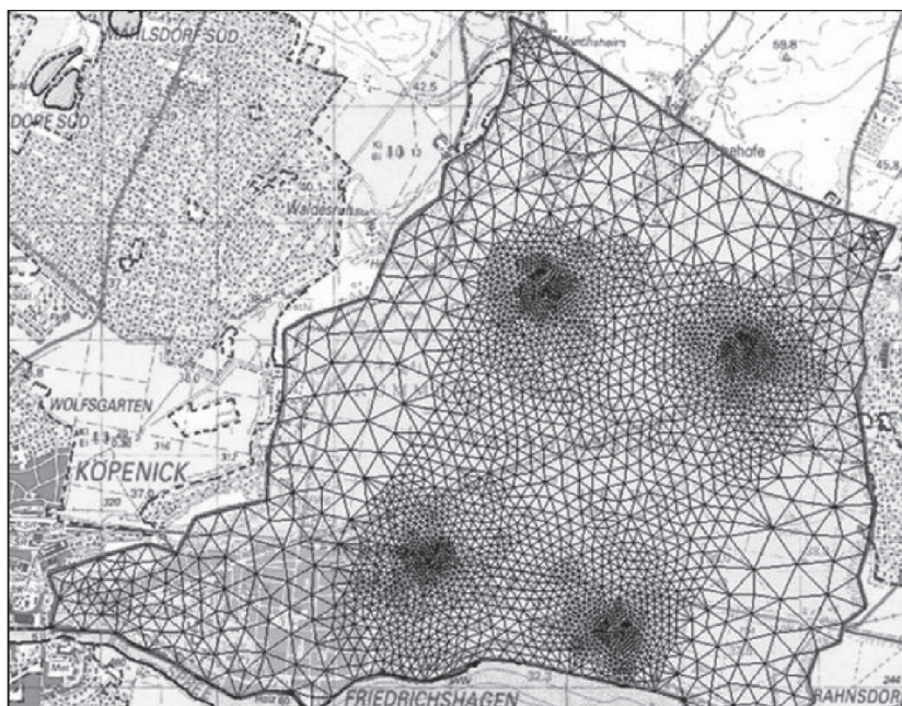
Fig. 15.11 Plan view of a finite element discretisation of an aquifer containing wells to simulate an aquifer remediation scheme. (From a FEFLOW test problem, Trefry and Muffels, 2007, with kind permission of John Wiley & Sons.)
