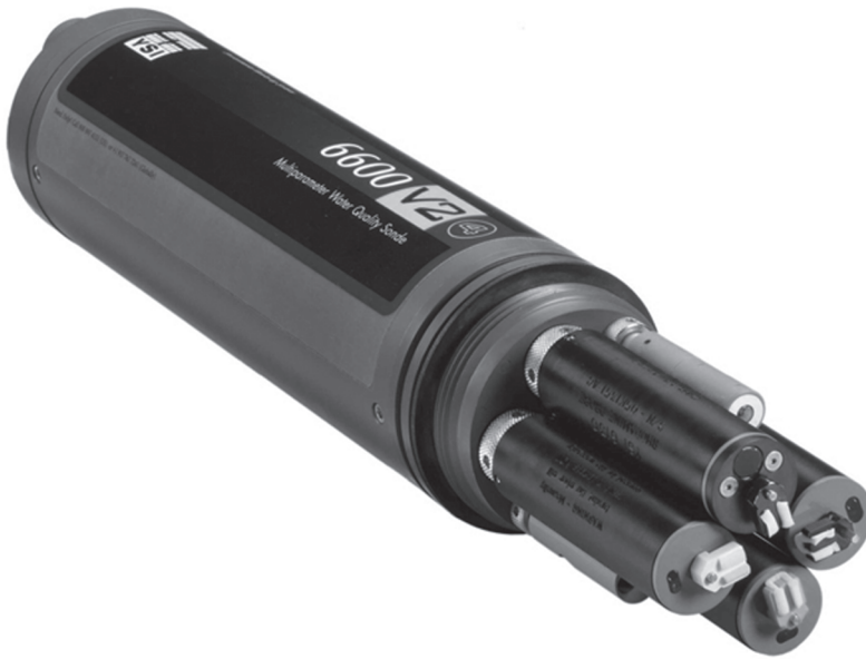
Fig. 8.6 A 6-series multi-probe sonde. (Reproduced by permission of YSI Inc., Yellow Springs, USA.)
