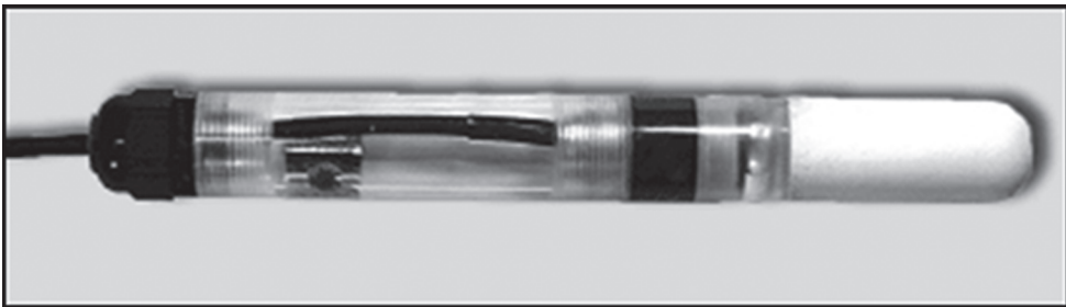
Fig. 6.6 A tensiometer with integral transducer. (Reproduced with permission of UMS GmbH)
